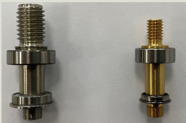
New tonearm bearing (left) and old tonearm bearing (right).
